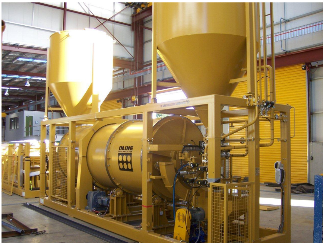
Figure 2: InLine Leach Reactor (ILR2000 model shown)
