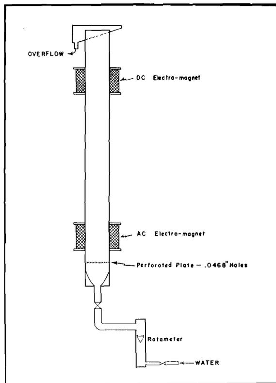
Fig. 1—Sketch of magnetic-reflux classifier for batch tests.
