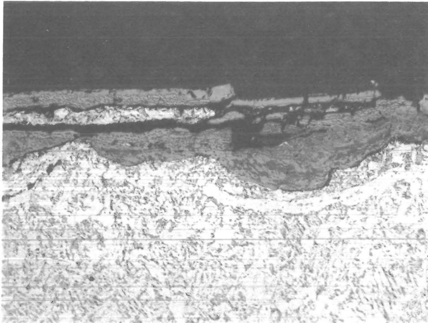
FIGURE 5. - Flaking of surface of steel ball (X 200) subjected to repeated impacts. Ball from alloy 1 after 530,000 impacts. Dark gray in upper region is plastic mounting material, gray near middle is oxidized iron, lower region is martensitic steel.
