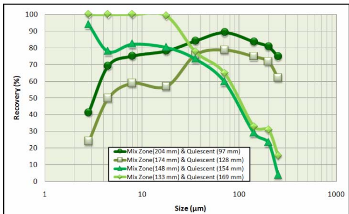
Figure 18. Recovery by size fraction, related with Quiescent and mix zones, Rotor X and Stator A at different Jg's, 1500 RPM
