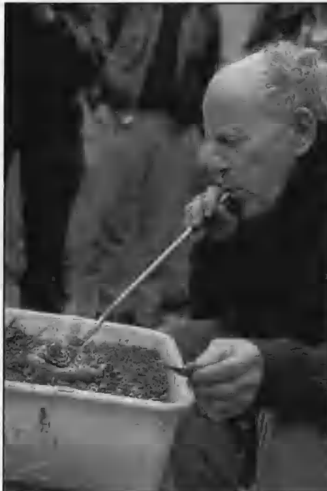
Bryan Earl smelting tin in the courtyard of the Oriental Institute
