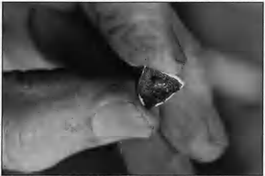
Tin prill smelted in courtyard of Oriental Institute fused to fragment of crucible
