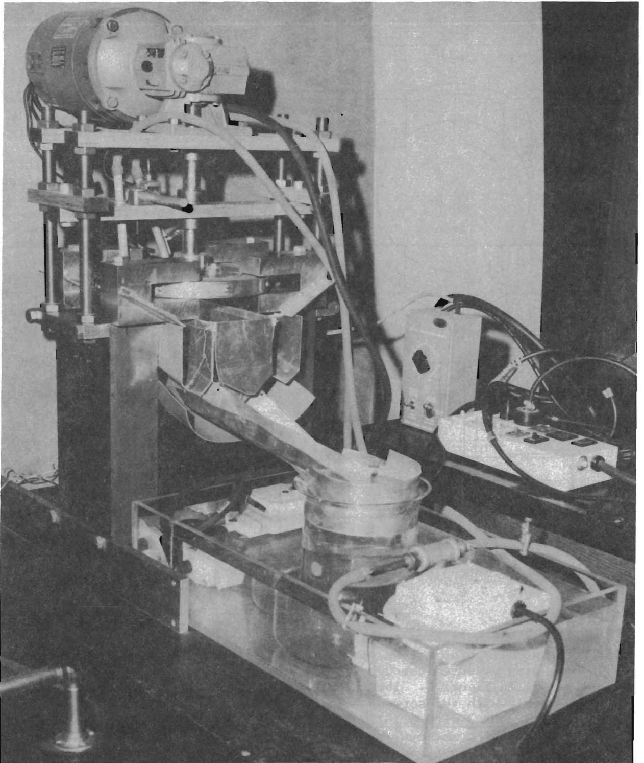
FIGURE 3. - Complete Separator With the Mechanical Drive Above the Matrix and the Magnetizing Coil Below the Discharge Launder.
