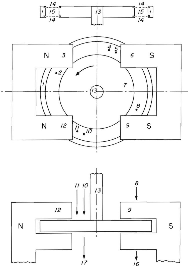
FIGURE 2. - Ring-Type Matrix Separator.
