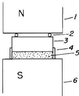
FIGURE 6. - Magnetic Circuit for Measuring Reluctance by a Substitution Method.
