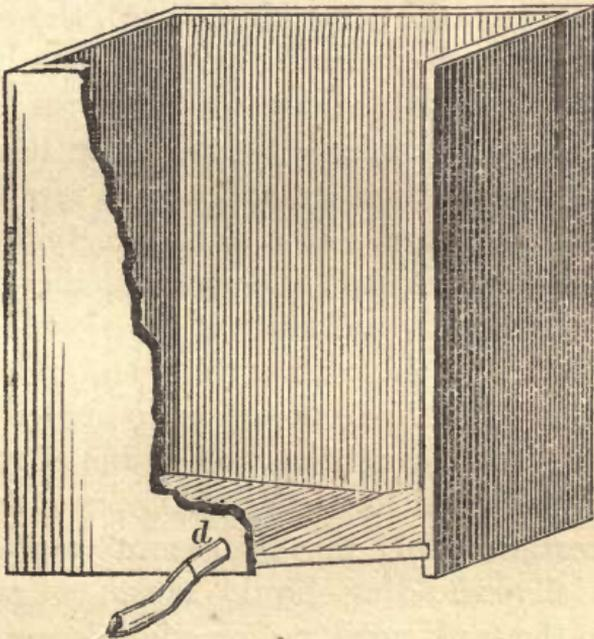
precipitating tanks, of which three or four are employed. If tubs are used, which for this purpose are the best, they are from three to four feet in diameter, and four feet high. The tanks or
