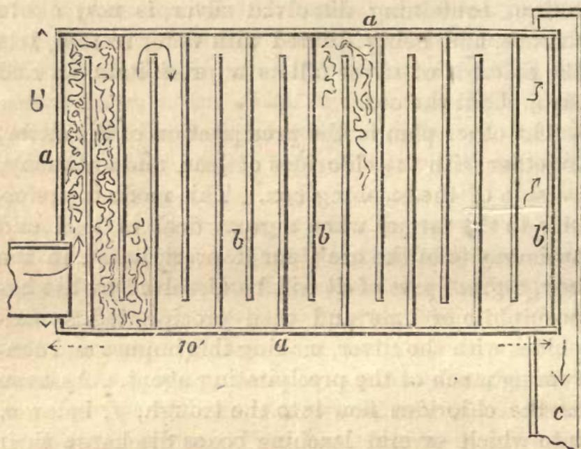
posit on. The fluid entering the trough, *c*, contains now a purified copper solution. Chloride of iron is also with the copper in solution, but does not prevent the copper from precipitating.
