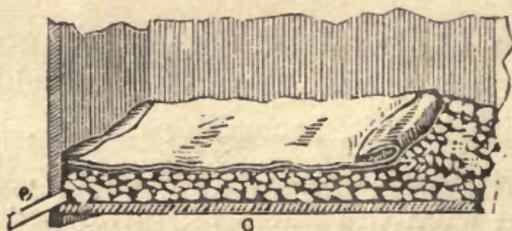
with numerous holes, one-half inch in diameter, about one inch above the bottom, *b*, or as Fig. 11 shows, without a false bottom. On the bottom, *a*, is thrown clean rock, quartz or poor ore of about the size of a hen's egg, three or four inches
