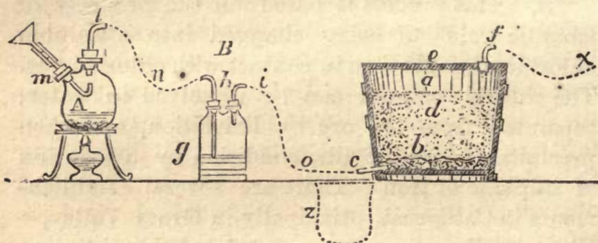
A common water bucket is then prepared to receive the moistened ore, which must not be too wet, but only moist enough to allow its being sifted. On the bottom of the bucket, *a*, Fig. 17, some clean rock or broken glass is placed about two inches deep, and covered with a piece of moistened canvas. A short glass pipe, *c*, two-eighths of an inch in diameter, is inserted close above the bottom.
