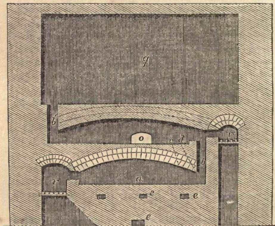
in Fig. 5, in longitudinal cross section. The lower hearth, *a*, is nine feet long and ten feet wide. The
