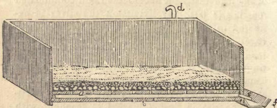
The boxes must be made as water-tight as possible and provided with a filter at the bottom. The filter is prepared in two ways, either as represented in Fig. 10 by fixing a false bottom, *a*, provided
