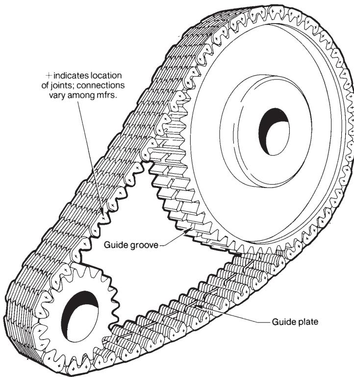
Figure 9 — Inverted tooth (silent) chain drive. These sprockets are grooved for center guide chain.
