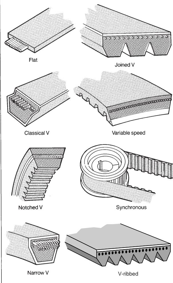
Figure 1 — Representative belt configurations.
