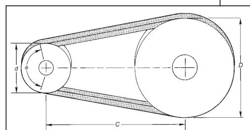
Figure 4 — Basic dimensions for calculating open and crossed belt lengths and arc of contact on smaller pulley or sheave.
