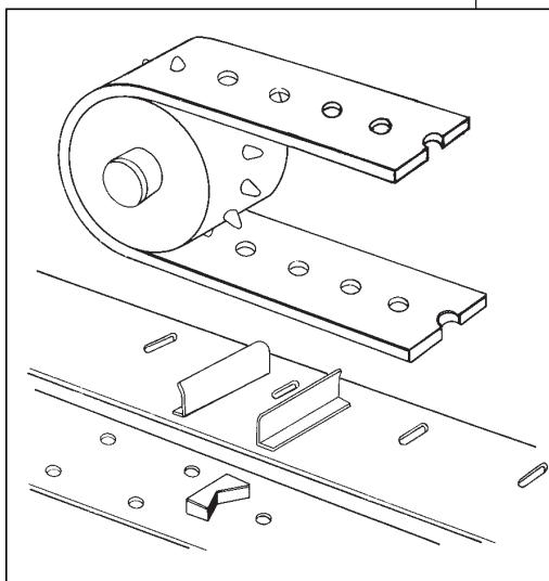
**Figure 5 — Metal belt attachments**
