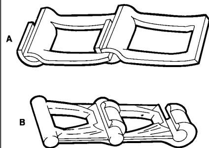
Figure 10 — Pressed steel detachable link chain, A, and malleable iron detachable link chain, B.
