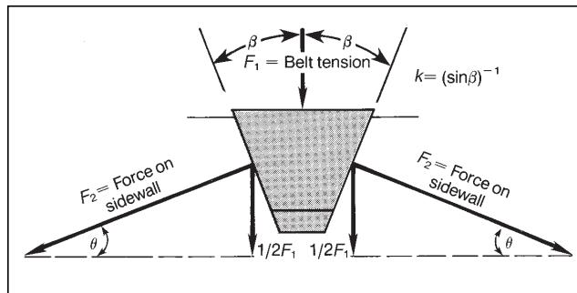
Figure 3 — Wedging action of V-belt increases force of belt against sheave groove and helps prevent slip.
