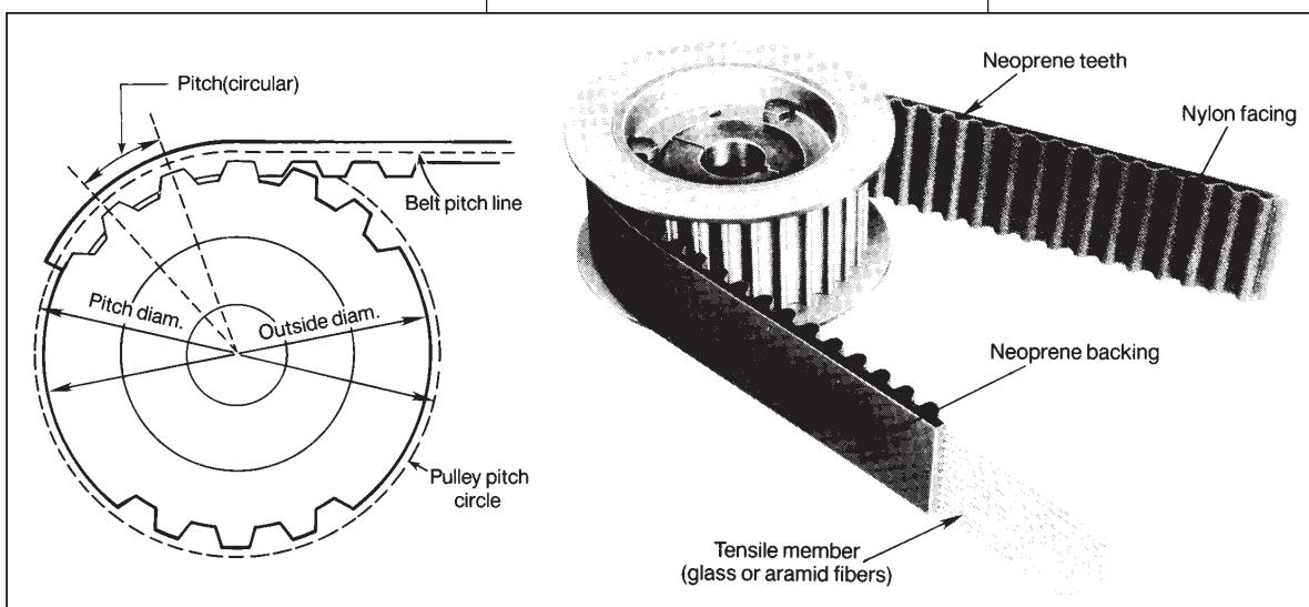
**Figure 6 — Typical synchronous belt and pulley with trapezoidal teeth, left, and curvilinear-tooth, high-torque drive, right.**
