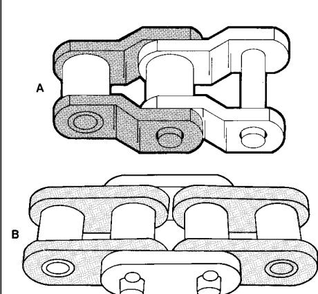
Figure 11 — Heavy duty, offset sidebar engineering steel roller chain, A, and heavy duty, straight sidebar roller type conveyor chain, B.
