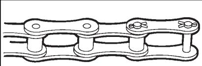
Figure 8 — Double pitch roller chain.
