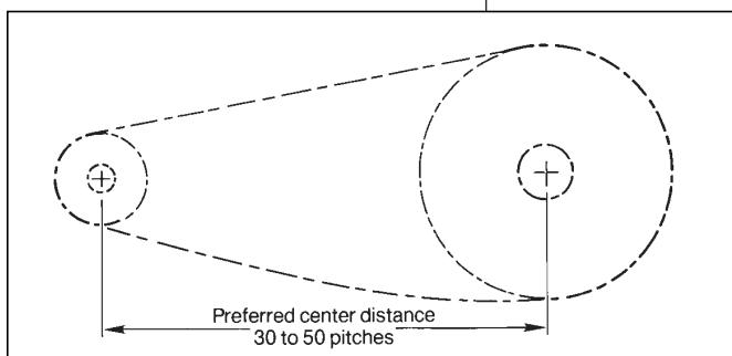
Figure 12 — Preferred range of center distance for roller chain drives.
