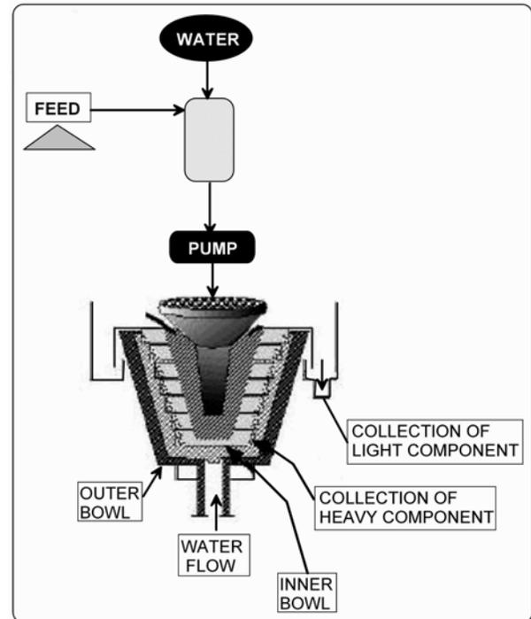
Fig. (1). Centrifugal gravity separator: A principal scheme.
