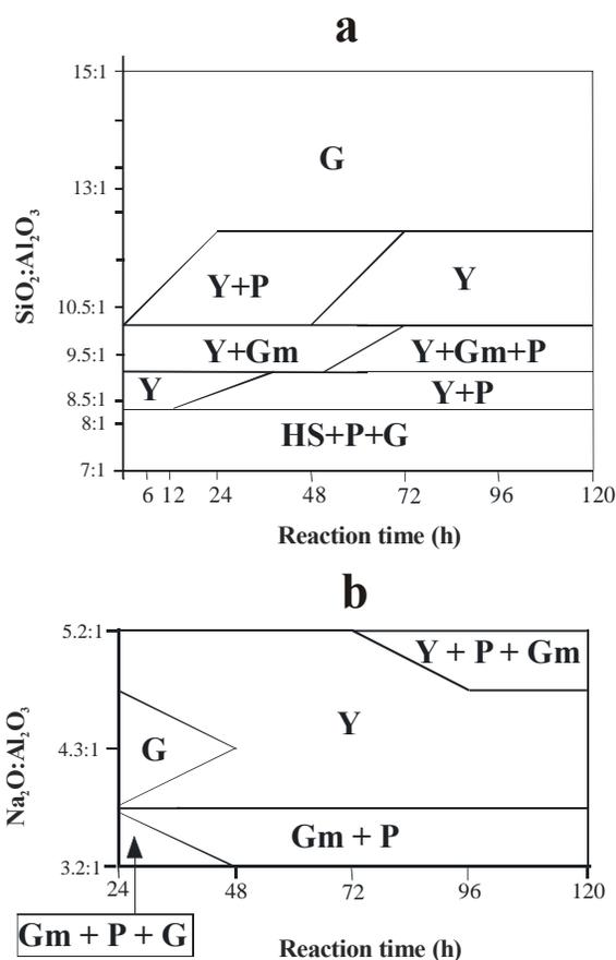
**Fig. (1).** Crystallization fields of the synthetic zeolites formed in the system: a) SiO<sub>2</sub>:Al<sub>2</sub>O<sub>3</sub>-time plot for a Na<sub>2</sub>O:Al<sub>2</sub>O<sub>3</sub> molar ratio of 4.2:1 and b) Na<sub>2</sub>O:Al<sub>2</sub>O<sub>3</sub>-time plot for a SiO<sub>2</sub>:Al<sub>2</sub>O<sub>3</sub> molar ratio of 10.5:1. Y= zeolite Y, P=zeolite NaP<sub>c</sub>, Gm=gmelinite-Na, HS=the OH-analogue of sodalite, G=amorphous material.
