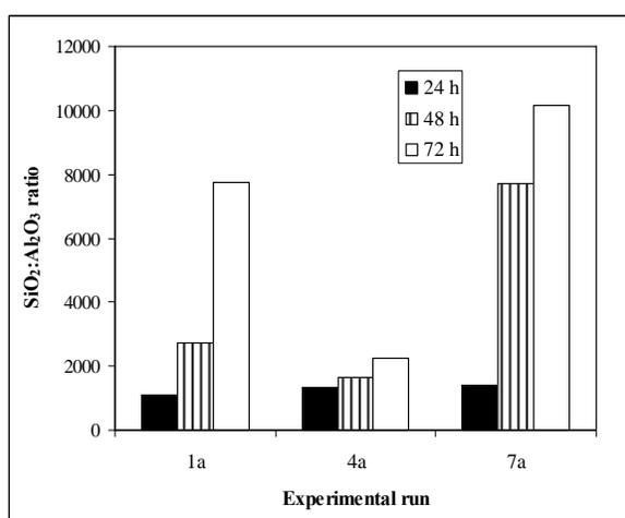
**Fig. (6).** Evolution of the  $\text{SiO}_2:\text{Al}_2\text{O}_3$  molar ratio in the fluid phase of the starting gel during crystallization of zeolite Y from  $\text{SiO}_2$ -sinter at various experimental runs. 1a, 4a, 7a= $\text{SiO}_2:\text{Al}_2\text{O}_3:\text{Na}_2\text{O}$  molar ratios of starting gel. 1a=10.5:1:4, 4a=10.5:1:5, 7a=10.5:1:3.
