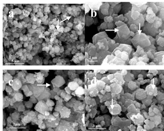
**Fig. (5).** SEM micrographs of zeolite Y end products produced from  $\text{SiO}_2$ -sinter. a) 48 h reaction time. The arrows indicate amorphous matter. b) 72 h reaction time. The arrows indicate crystals with octahedral habit. c) 97 h reaction time. The arrow indicates zeolite Y twins. d) 120 h reaction time. The arrows indicate the formation of growth spirals on the surface of zeolite Y
