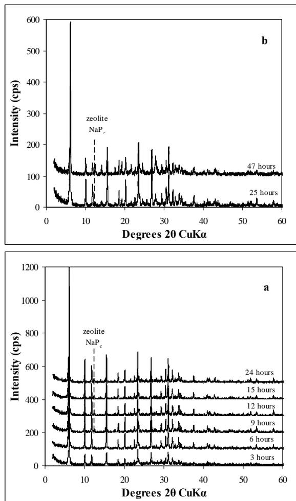
**Fig. (2).** XRD diagrams showing zeolite Y synthesized a) from SiO<sub>2</sub>-rich sinters and b) from perlite.
