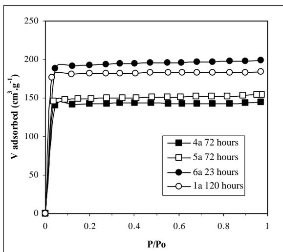
**Fig. (4).** Adsorption isotherms of the synthetic zeolites. 1a, 4a, 5a, 6a=  $\text{SiO}_2:\text{Al}_2\text{O}_3:\text{Na}_2\text{O}$  molar ratios of starting gel. 1a = 10.5:1:4, 4a= 10.5:1:5, 5a=9.5:1:4, 6a=8.4:1:4.
