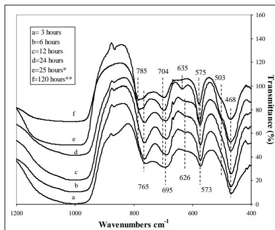
**Fig. (3).** FTIR spectra of synthetic zeolite Y, a-d= from SiO<sub>2</sub>-sinter and SiO<sub>2</sub>:Al<sub>2</sub>O<sub>3</sub> ratio 8.4:1, e= from perlite and SiO<sub>2</sub>:Al<sub>2</sub>O<sub>3</sub> ratio 8.4:1, f= from SiO<sub>2</sub>-sinter at SiO<sub>2</sub>:Al<sub>2</sub>O<sub>3</sub> ratio 10.5:1.
