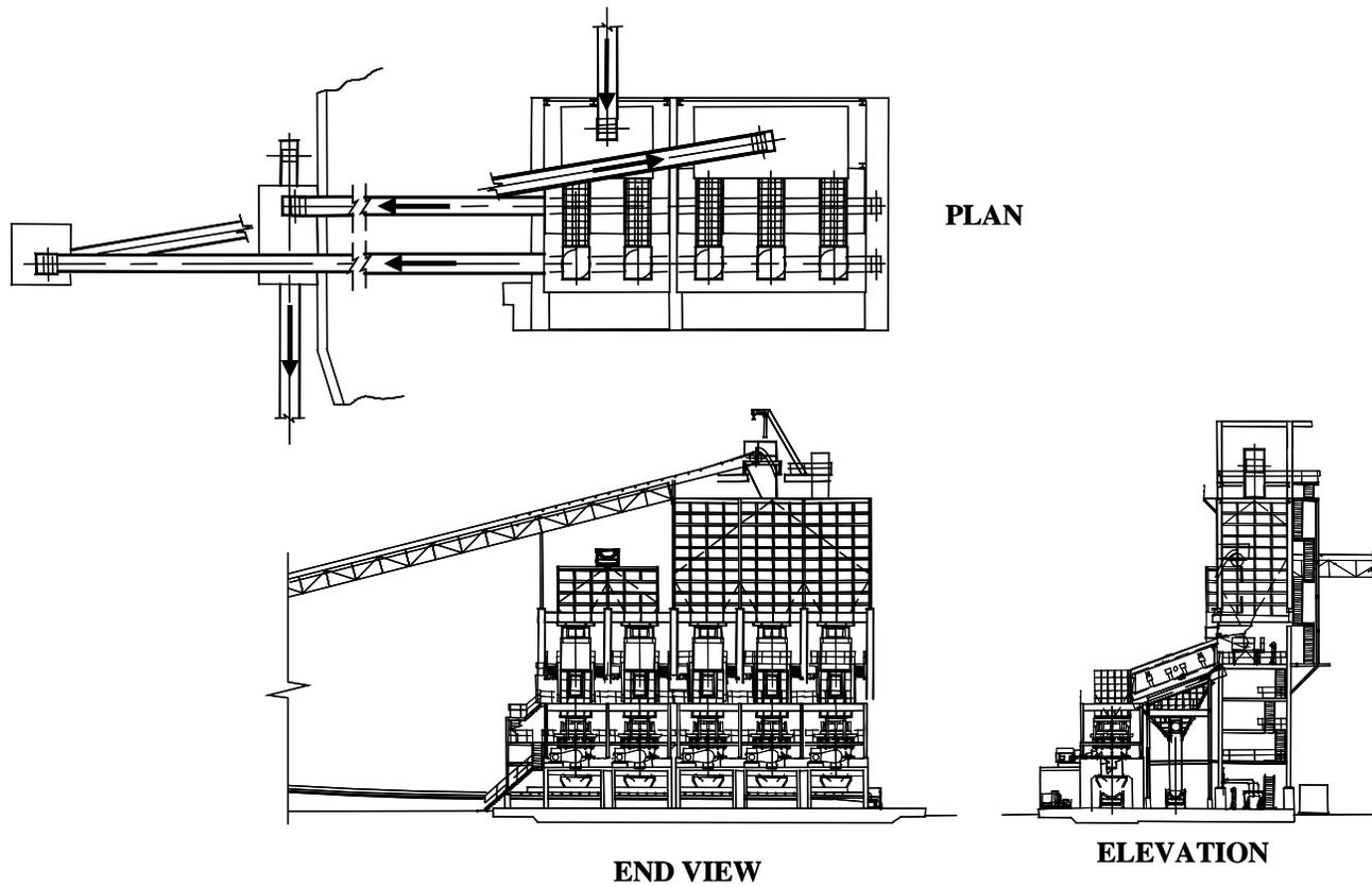
Figure 19 Typical secondary and tertiary closed circuit layout
