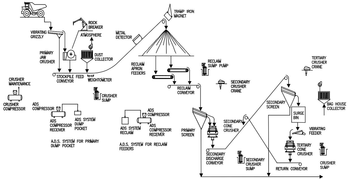
Figure 6 Three stage crushing closed circuit
