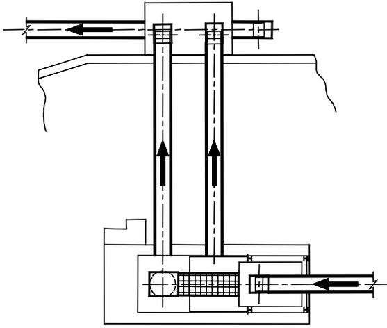
Figure 13 Open circuit (1) secondary crusher
