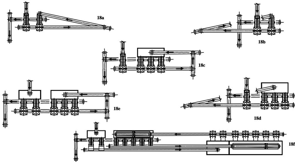
**Figure 18 Typical closed circuit secondary and tertiary crushers**
