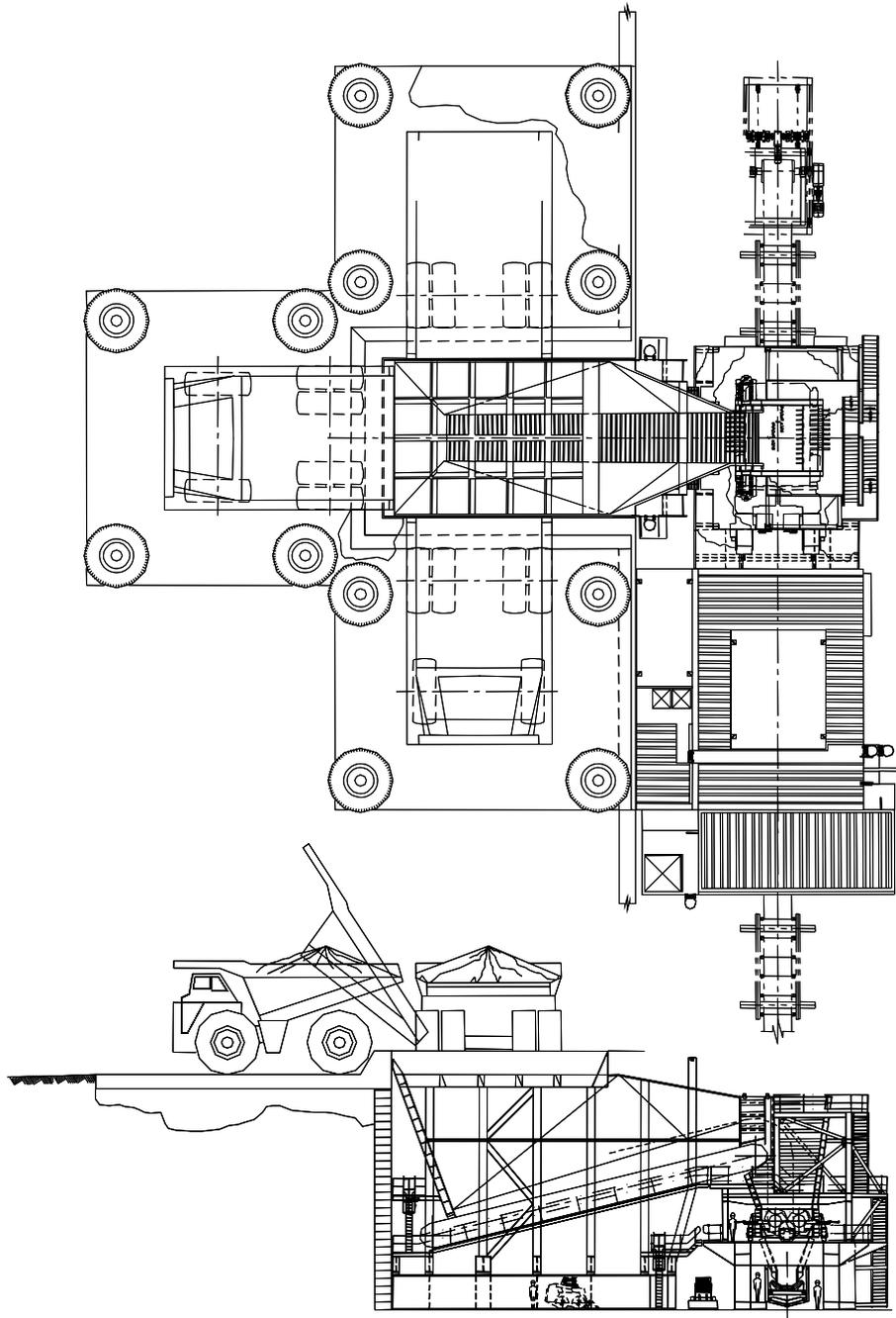
**Figure 12 Typical low speed roll sizer installation**
