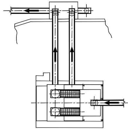
Figure 14 Open circuit (2) secondary crushers
