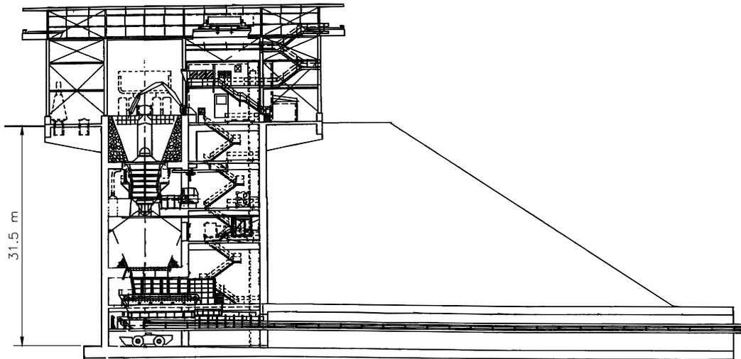
**Figure 8 60' x 89' gyrotory installation, Freeport, Indonesia**
