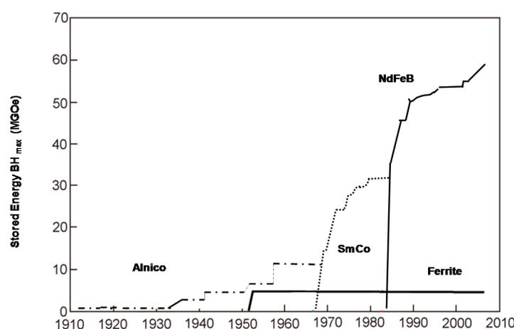
**Figure 11.** Development of permanent magnets, modified from [48]. The  $y$ -axis is the magnet performance, expressed as stored energy  $(BH)_{\max}$ , measured in units of megagauss-oersted (MGOe).
