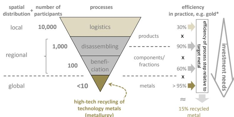
**Figure 13.** Process chain of recycling for consumer goods: technology metals from printed circuit boards [60].
