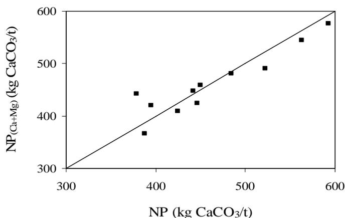
Figure 4. Calculated NP<sub>(Ca+Mg)</sub> vs. measured NP of the different waste rock size fractions
