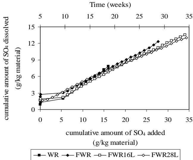
Figure 8. Cumulative amount of  $\text{SO}_4$  dissolved vs. the cumulative amount of  $\text{SO}_4$  introduced in the waste rock humidity cells
