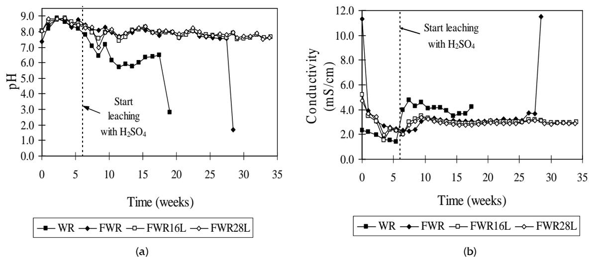
Figure 5. Variation of (a) pH and (b) conductivity vs. time in the leachates of waste rock and limestone amended humidity cells
