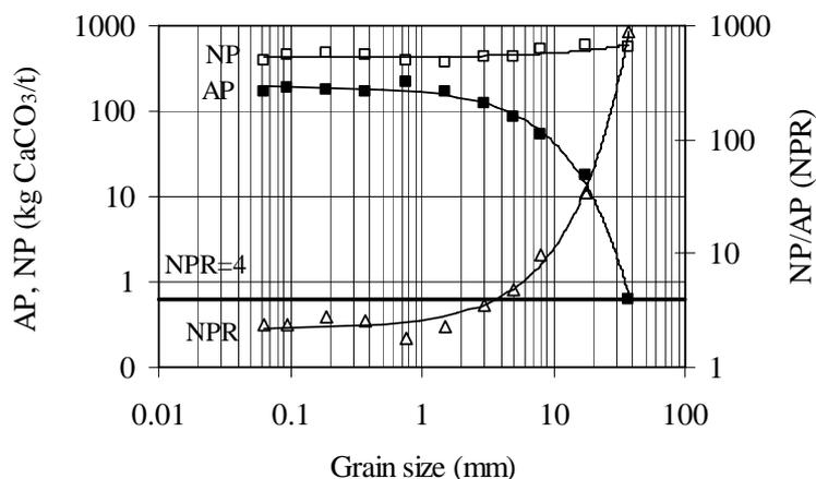
Figure 3. AP, NP and NPR vs. particle size of the waste rock material
