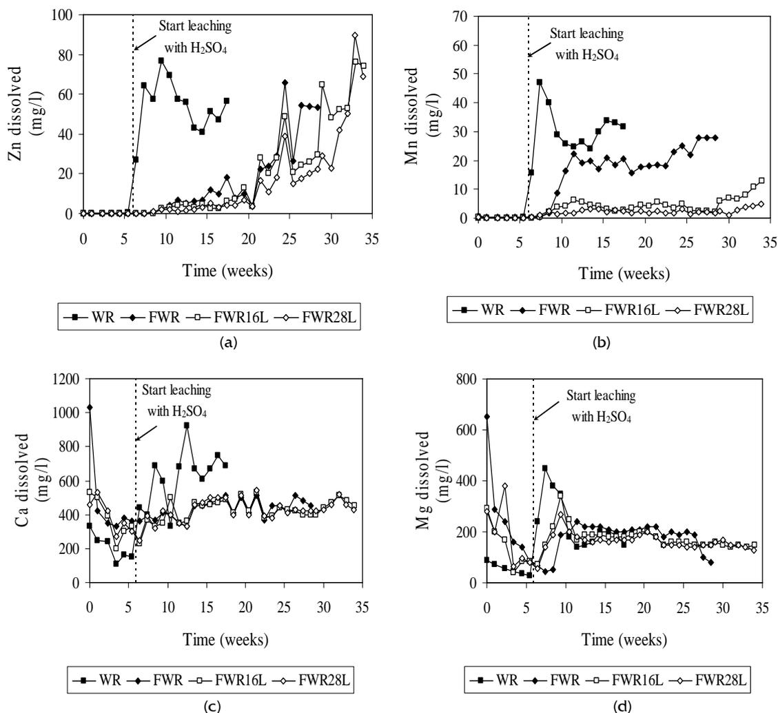
Figure 6. Variation of (a) Zn, (b) Mn, (c) Ca and (d)mg dissolved concentrations in the leachates of waste rock humidity cells
