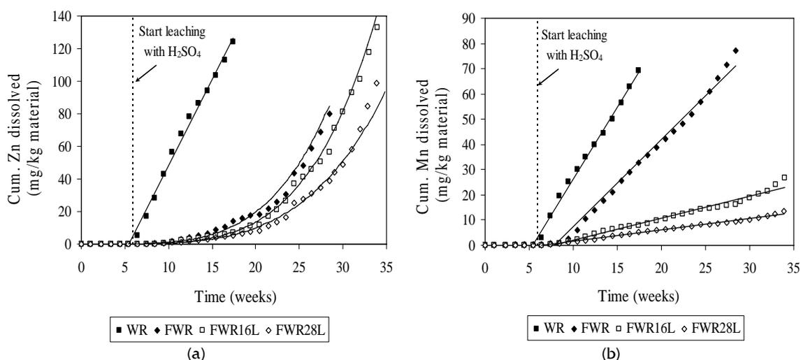
Figure 7. Cumulative amount of (a) Zn and (b) Mn dissolved in the leachates of the waste rock humidity cells
