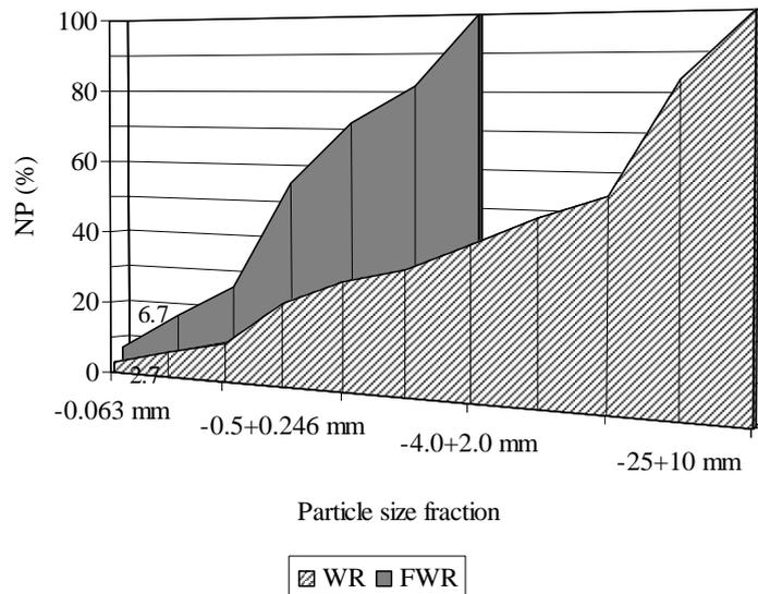
Figure 9. Contribution of the different size fractions to the NP value of the whole waste rock sample (WR) and the -4mm size fraction (FWR)
