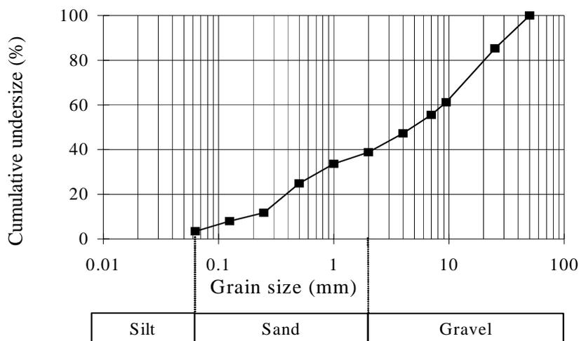
Figure 2. Particle size distribution of Stratonis waste rock sample
