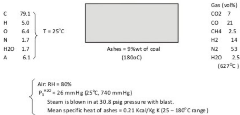
**Figure 37.2: Material balance diagram**
