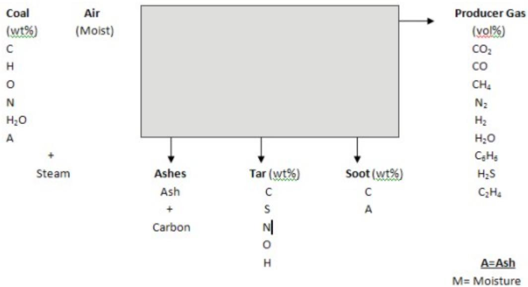
**Figure 37.1: Material balance in gasification**
