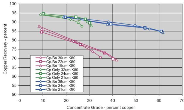
FIG 4 - Results from batch cleaner tests – copper grade recovery curves.
