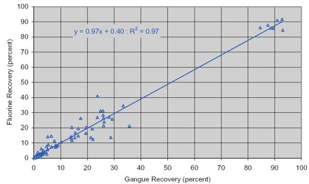
FIG 2 - Relationship between non-sulfide gangue recovery and fluorine recovery to copper concentrate.
