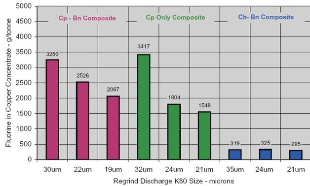
FIG 3 - Effect of regrinding on fluorine content of copper concentrate.
