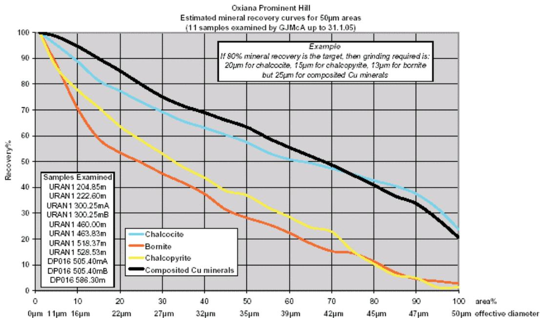
FIG 1 - Estimated copper mineral recovery versus sizing.
