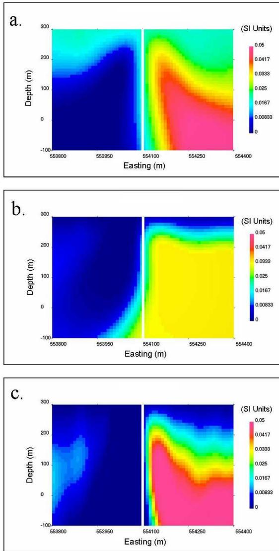
**Figure 4:** Inversion results for the faulted contact model after manipulation of inversion parameters. a) Reference model set to 0.02 SI Units (default value is 0 SI Units); b) Bounds set from 0 to 0.035 SI Units (default bounds are from 0 to 1 SI Units); c)  $z$  and  $y$  increased relative to  $x$  ( $z = y = x$  for default inversion).
