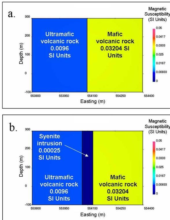
**Figure 2:** Cross-sections looking north through 3D magnetic susceptibility models associated with a) the faulted contact model, and b) the syenite intrusive model. Depth in m on the vertical axis and distance in UTM (m) on the horizontal axis.
