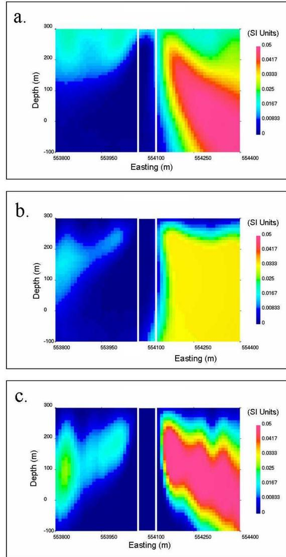
**Figure 5:** Inversion results for the faulted contact model after manipulation of inversion parameters. a) Reference model set to 0.02 SI Units; b) Bounds set from 0 to 0.035 SI Units; c)  $z$  and  $y$  increased relative to  $x$ .
