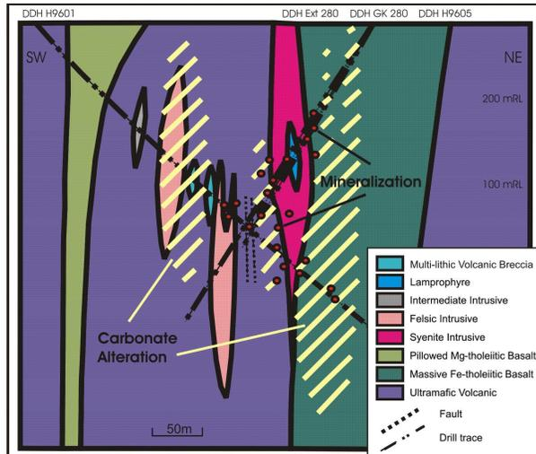
**Figure 1:** Cross-section, facing northwest, through the Hislop gold deposit, showing carbonate altered, and mineralized rocks.
