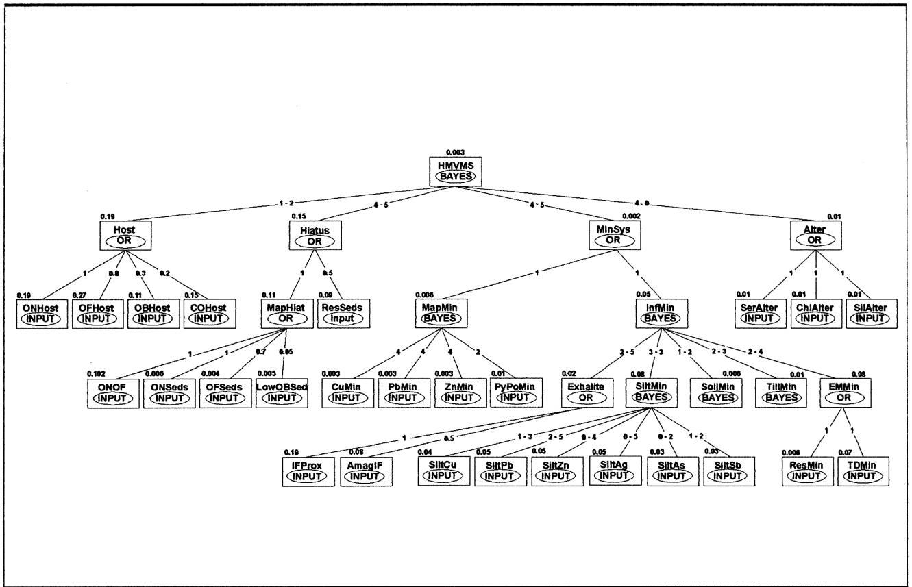
Figure 2: Inference network of the Halfmile Lake volcanogenic massive sulphide deposit model used in the Bathurst geographic expert system (GES) study.
