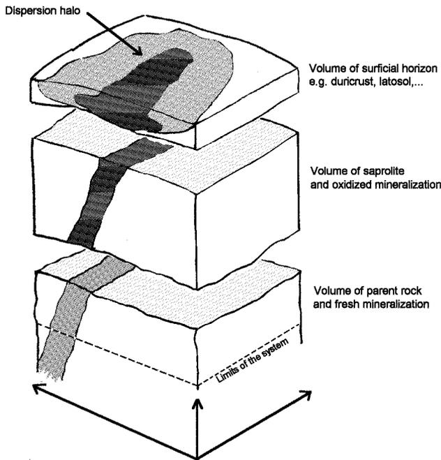
**Figure 2:** Sketch of the system taking into account the volumes for the gold mass balance calculation.
