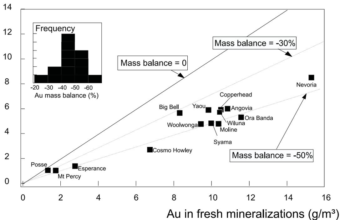
**Figure 4:** Distribution of the average Au mass content in the oxidized saprolite versus that in the fresh parent rock for various mineralized lateritic deposits (including a bar chart of the gold mass balances).
