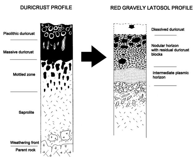
**Figure 1:** Schematic ferruginous duricrust profiles and their transformation to red gravelly latosols.
