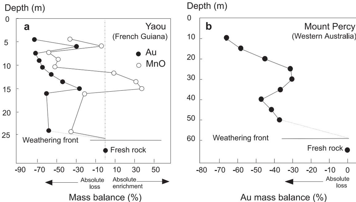
**Figure 3:** Gold mass balance in the saprolite profile of the Yaou (a) and the Mount Percy deposits (b). The reference is the average gold content in the parent rock.
