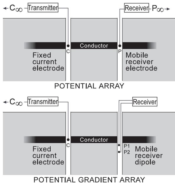
**Figure 1:** Electrode configurations in borehole mise-à-la-masse potential and potential gradient measurements.
