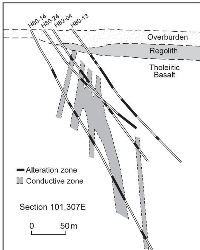
**Figure 10:** Conductivity structure between H82-04 and H80-14 interpreted from the *mise-à-la-masse* and resistivity logs.
