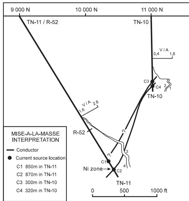
**Figure 16:** Interpretation of the mise-à-la-masse data between TN-11 and TN-10. Electrical continuity was established between nickel mineralisation in the two holes.
