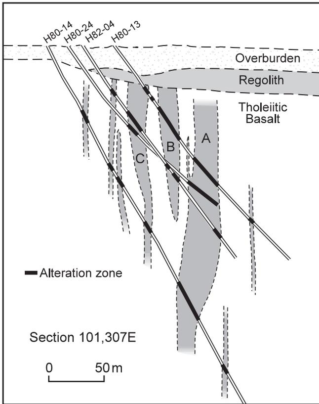
**Figure 7:** Geological cross-section along grid line 101,307E, Hoyle Pond Deposit. The alteration zones identified in the drill core are indicated as black shaded zones.
