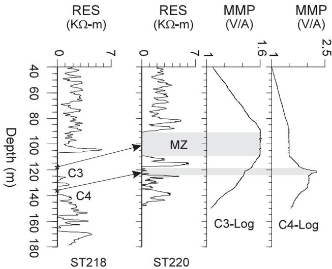
**Figure 12:** *Mise-à-la-masse* measurements acquired in ST220 with current sources in ST218. The C3- and C4-Logs represent potential-depth profiles with electrodes at C3 and C4, respectively. MZ = Main zone.
