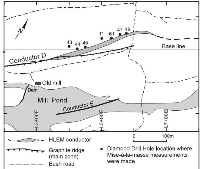
**Figure 3:** The D-zone, Victoria Graphite deposit, and location of holes where mise-à-la-masse measurements were made.
