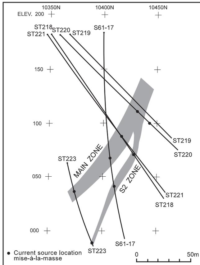
**Figure 11:** Geological cross-section of the Stratmat deposit (unpublished data, courtesy Noranda Exploration Ltd.).
