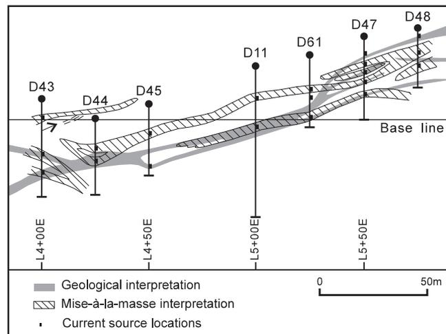
**Figure 6:** Plan view showing a comparison between the geological and *mise-à-la-masse* interpretations of the D-zone.
