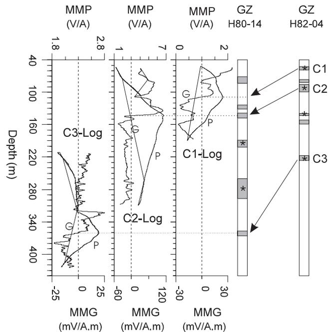
**Figure 9:** Mise-à-la-masse potential and gradient data acquired in H80-14 with the current electrodes in H82-04. C1-, C2- and C3-Logs represent measurements with the current electrodes at C1, C2 and C3, respectively. The arrows between the geologic columns represent the dominant current flow path.
