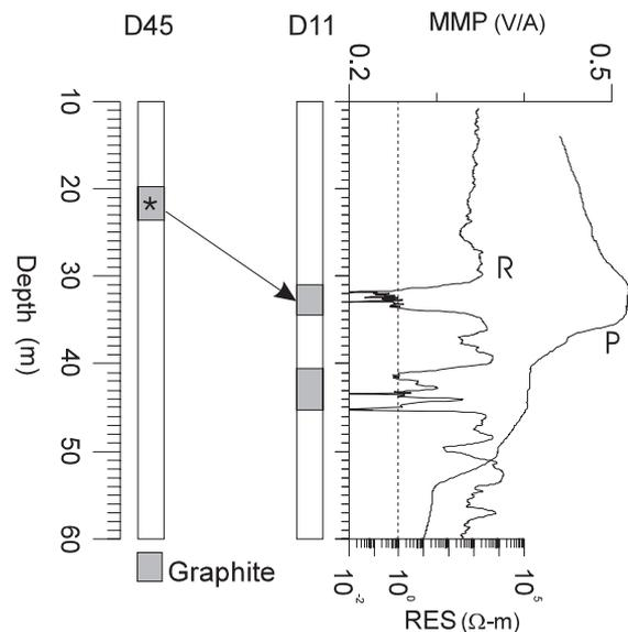
**Figure 4:** Resistivity and mise-à-la-masse potential logs from D11 with the current source located in the graphite zone in D45. A potential maximum across the upper graphite intersection indicates electrical connection with the energised zone in D45. The lower graphite zone shows a lower, flattened potential interval across it, characteristic of the response of an isolated conductor.
