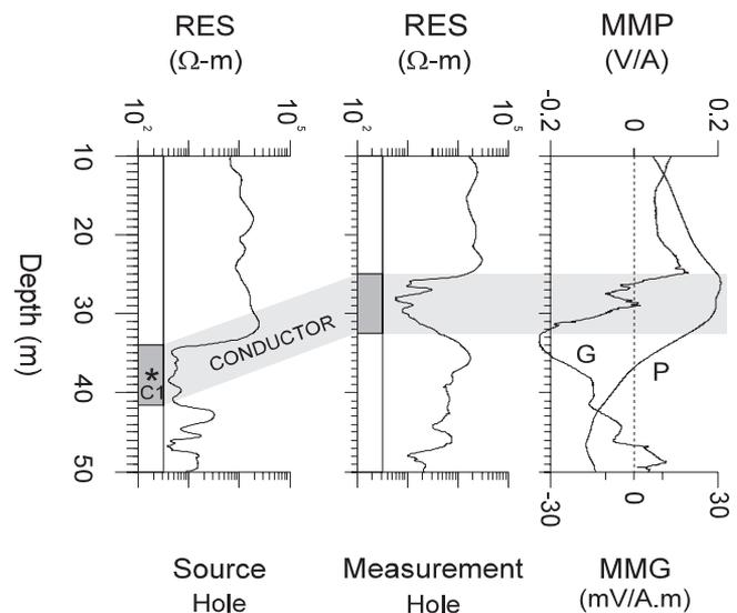
**Figure 2:** Field example showing the use of mise-à-la-masse potential (MMP) and potential (MMG) gradient measurements to establish continuity of conductive zones between boreholes. RES = resistivity, P = potential; G = gradient.
