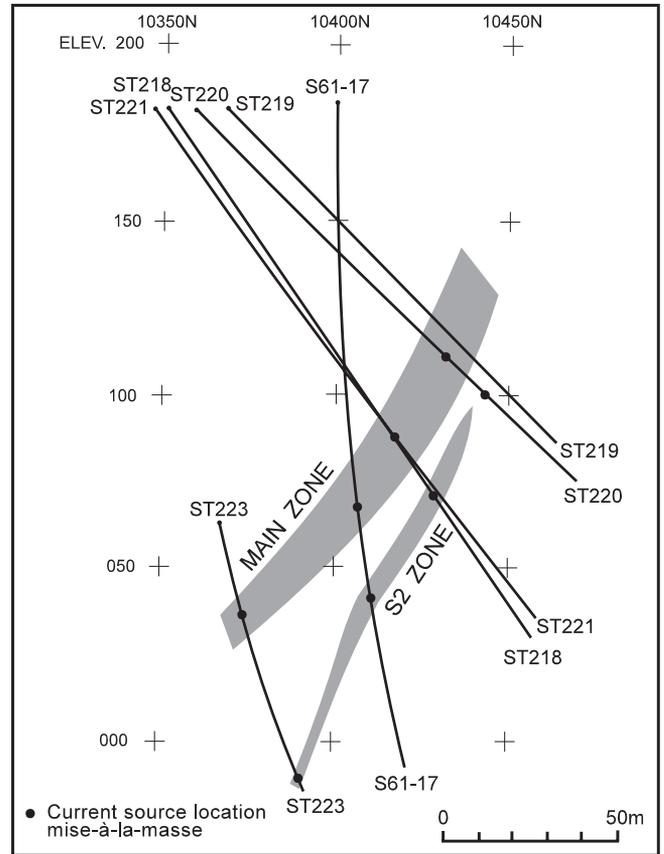
**Figure 14:** *Mise-à-la-masse* interpretation of the structure and geometry of the Stratmat deposit. The Main zone and the S2 zones are not connected.
