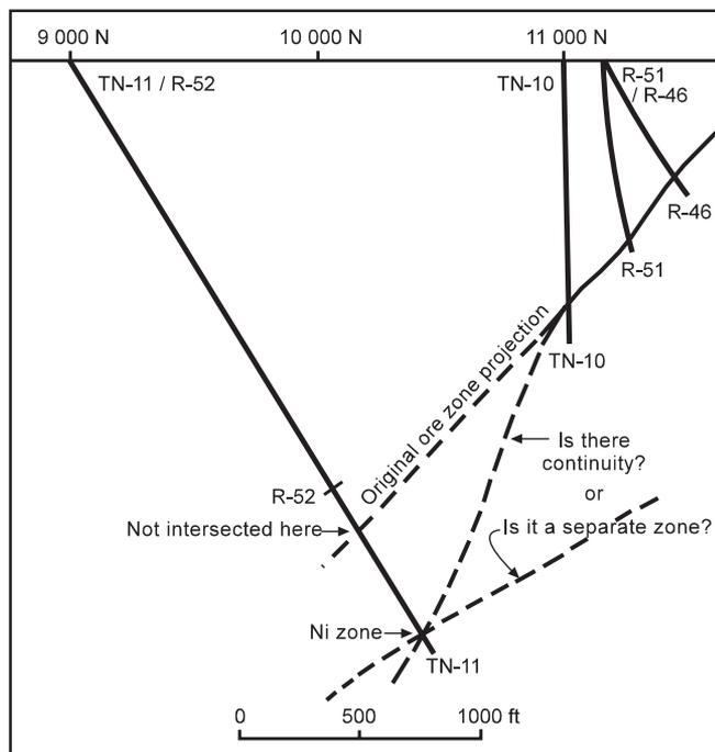
**Figure 15:** Geological problem presented at the Redstone nickel deposit, Timmins. Borehole TN-11 intersected nickel sulphides at a much greater depth than predicted by projecting the deposit orientation from the near-surface R-zone.
