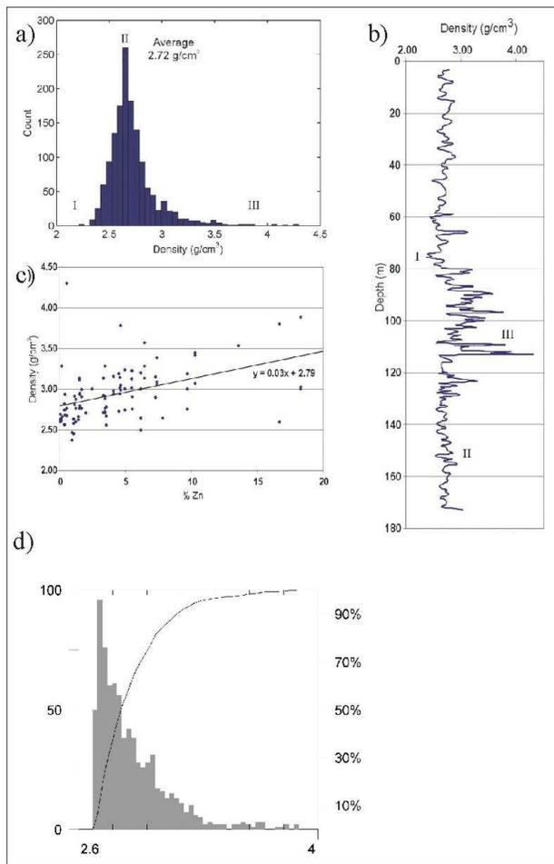
Figure 2: a) Density distribution from the measurements done on core; b) density log from one borehole. See text for details on the zones I, II and III; c) density vs. %Zn from one of the boreholes surveyed. Notice the linear relationship; d) cumulative histogram of all the density measurements, including those collected on core and those recovered from geochemical assays. Mean and median of density are 2.91 and 2.84  $\text{g}\cdot\text{cm}^{-3}$  respectively.
