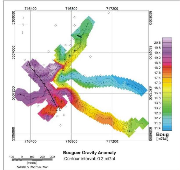
**Figure 4:** Bouguer gravity anomaly over the area of study. Location of profile AA' (model) is shown for reference. Borehole locations are showed as black circles/
