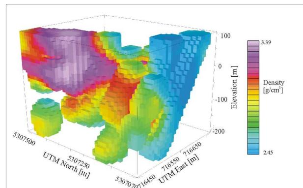
Figure 3: 3D density model over the area of study. Voxel cell size: 10 m.
