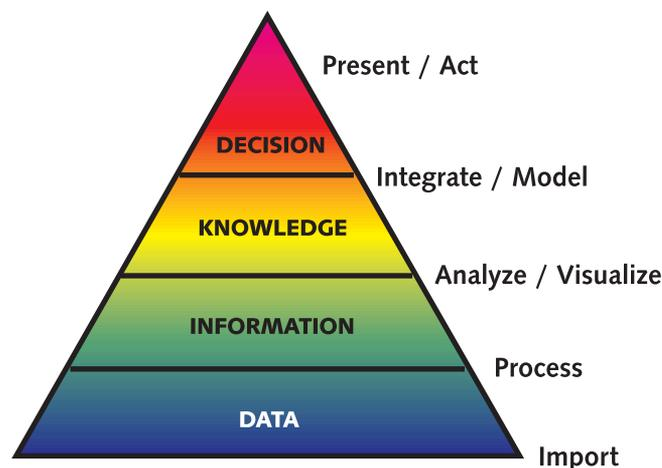
**Figure 2:** The DPA representation incorporates both the ESIP model and the subset of activities performed within a DPA software environment. The five activities to the right of the figure constitute the DPA Data Stream in which raw data is transformed to information, knowledge and decisions through specific computer-assisted tasks.
