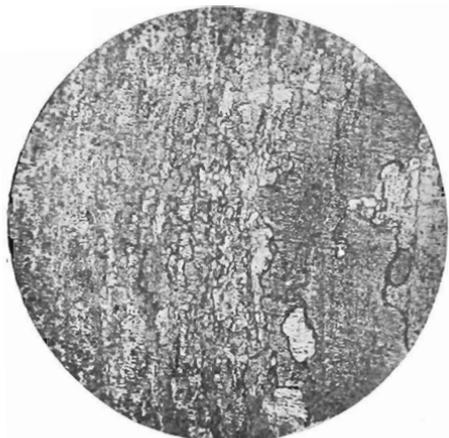
FIG. 43.—SWAGED TUNGSTEN ROD, 0.080 IN. DIAM., CONTAINING 0.75 PER CENT.  $\text{ThO}_2$ . HEATED  $9\frac{3}{4}$  HR. AT  $3000^\circ\text{C}$ . COLD END NEAR ELECTRODE CLAMP.  $\times 155$ .
