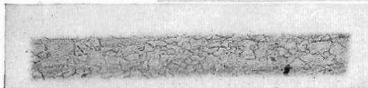
FIG. 48.—TUNGSTEN WIRE, 0.007 IN. DIAM., CONTAINING 0.75 PER CENT.  $\text{ThO}_2$ . RECRYSTALLIZED BY SHORT HEATING AT ABOUT  $2000^\circ\text{C}$ .  $\times 130$ .
