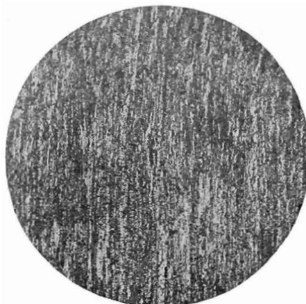
FIG. 38.—STRUCTURE OF SWAGED TUNGSTEN ROD, 0.80 IN. DIAM.  $\times 240$ .
