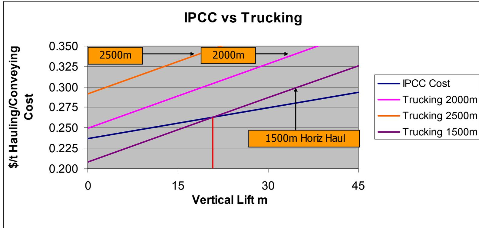
1. This graph shows when IPCC starts to produce lower operating costs versus truck haulage with horizontal haul distance ex-pit.
