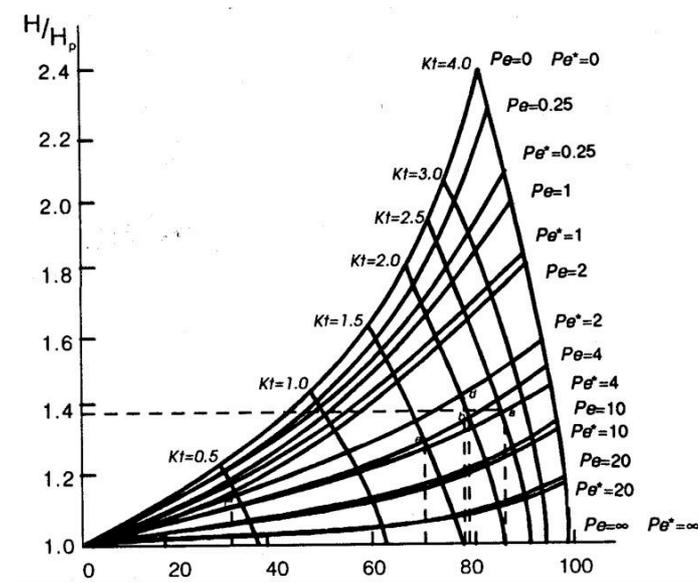
Figure 3. Modified diagram for evaluation of collection zone height based on axial dispersion equation (mass transfer model) and first-order kinetics (flotation model).
