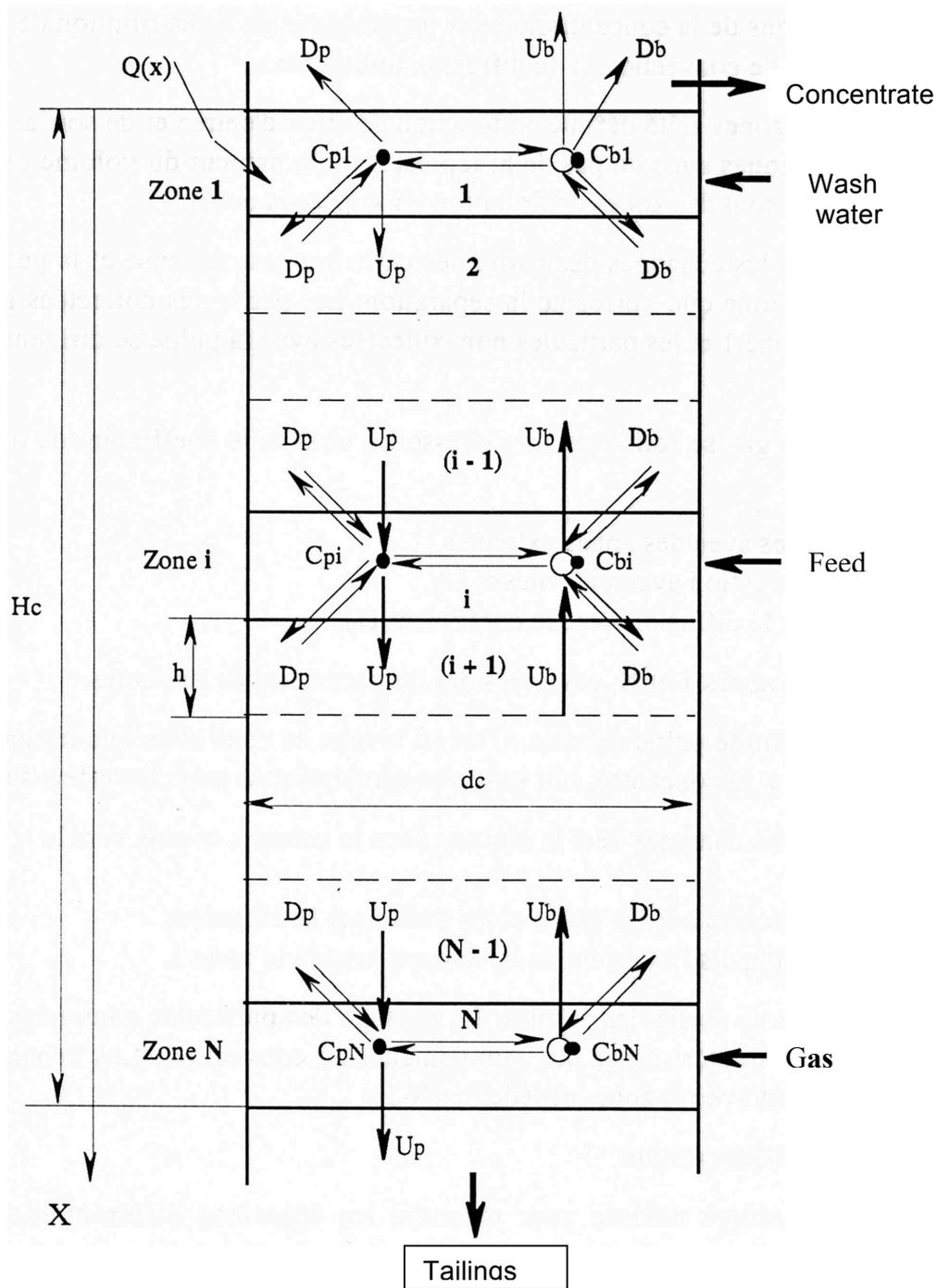
Figure 4. Diagram of transfers in collection zone and connections to external zones.  $H_c$  is the height of the collection zone,  $d_c$  is the column diameter,  $Q(x)$  is the particle flow from froth back to the slurry.
