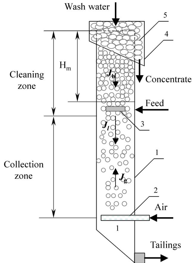
Figure 1 Diagram of column flotation: 1-column body, 2-sparger, 3-feed distributor, 4- froth launder, 5-froth.
