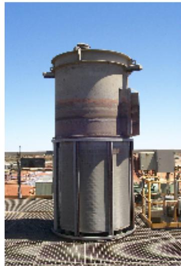
The screens will also become pegged with near sized carbon and other material such as small rocks and need to be removed and cleaned/replaced regularly to prevent tank overflows.
